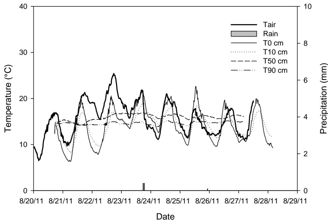
Figure 1. Meteorological and soil temperature data recorded during the field experiment.
