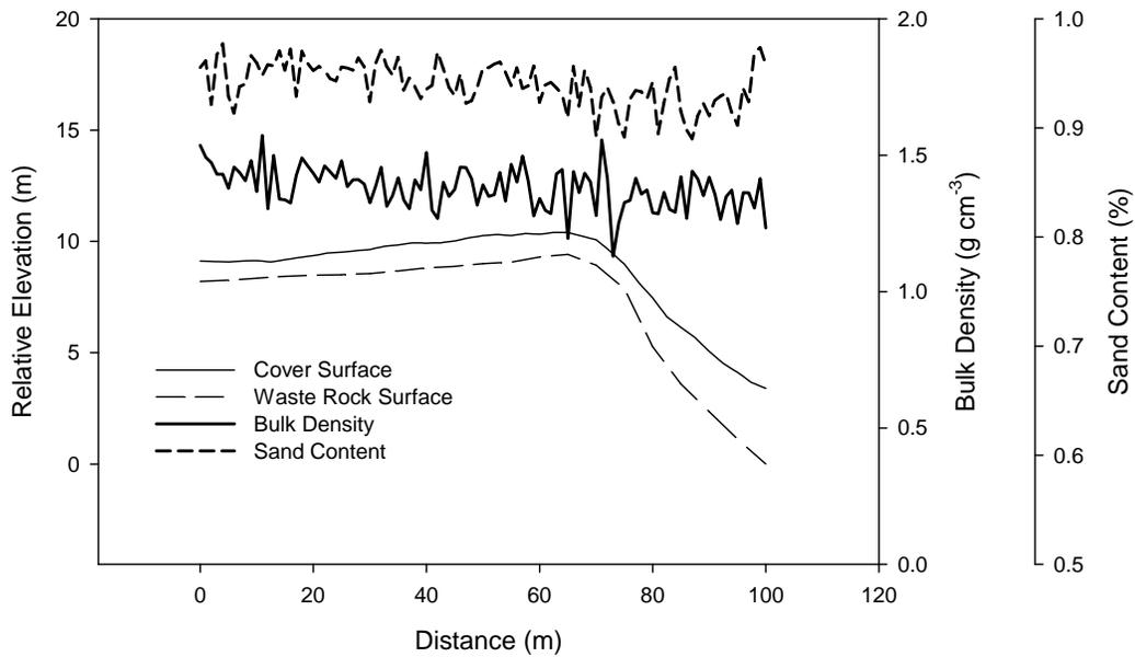
Figure 2. Spatial variation of bulk density, sand content, and relative elevation profile of the cover system experimental transect.
