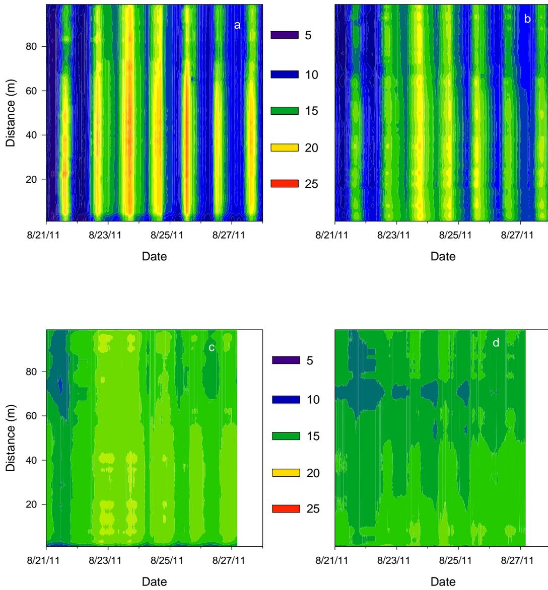
Figure 3. Distributed soil temperature values for the field experiment measured at a) 0, b) 10, c) 50, and d) 90 cm depths.
