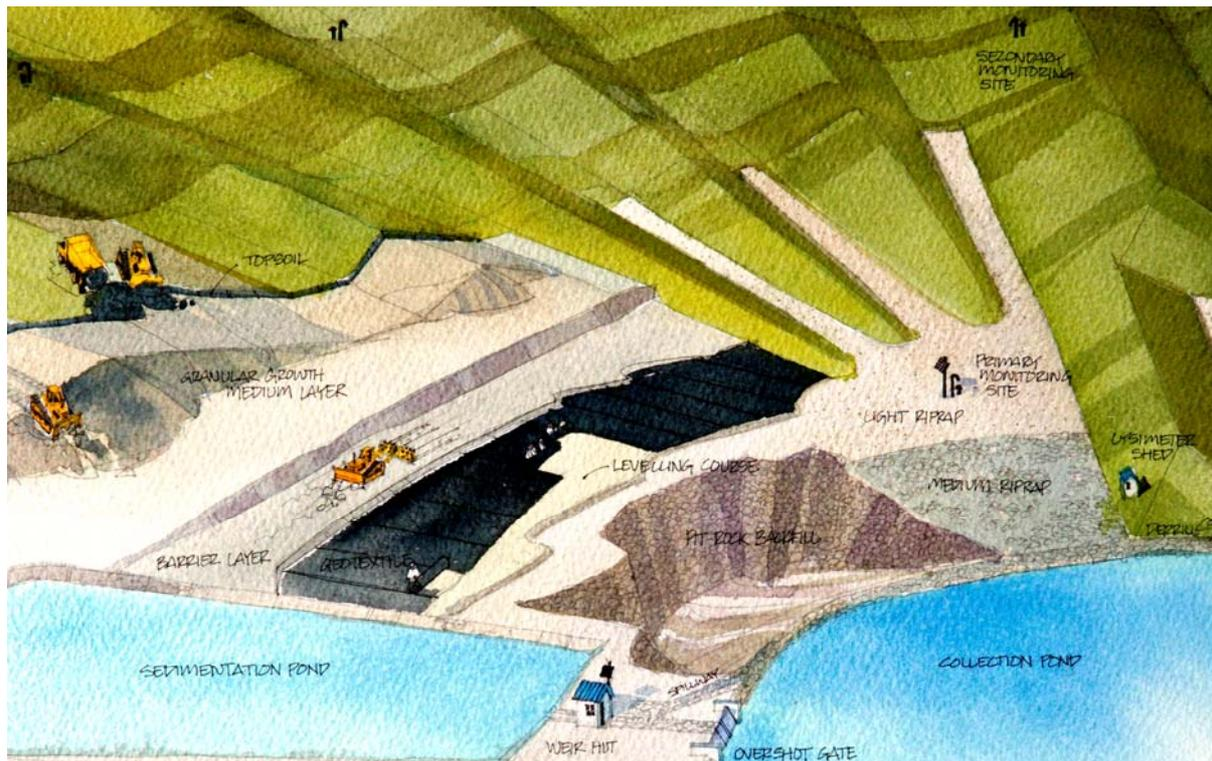
Figure 9. Rendering of the second landform alternative and key components for the pit cover system (from OKC, 2004).
