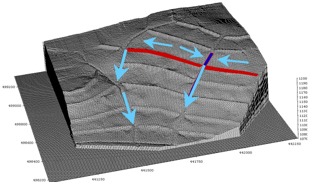
Figure 7. Surface contours (vertically enhanced) for the first landform alternative evaluated for the pit cover system (from OKC, 2004).
