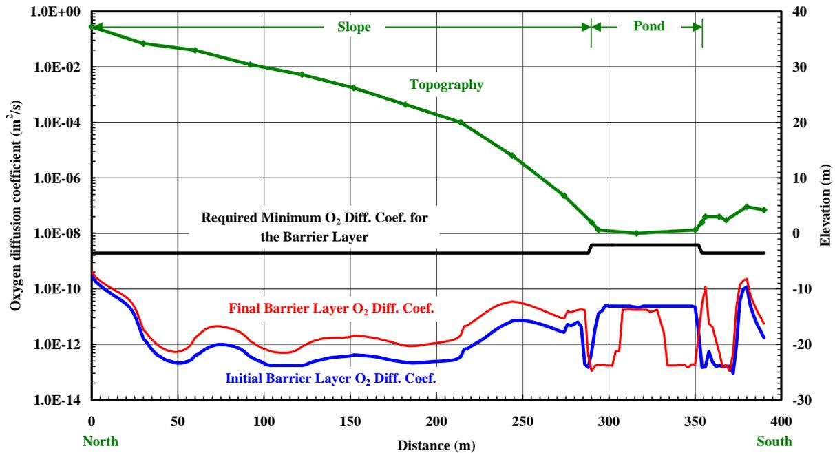
Figure 5. Initial and final predicted oxygen diffusion coefficient for the barrier layer assuming dry climate year conditions (from OKC, 2004).
