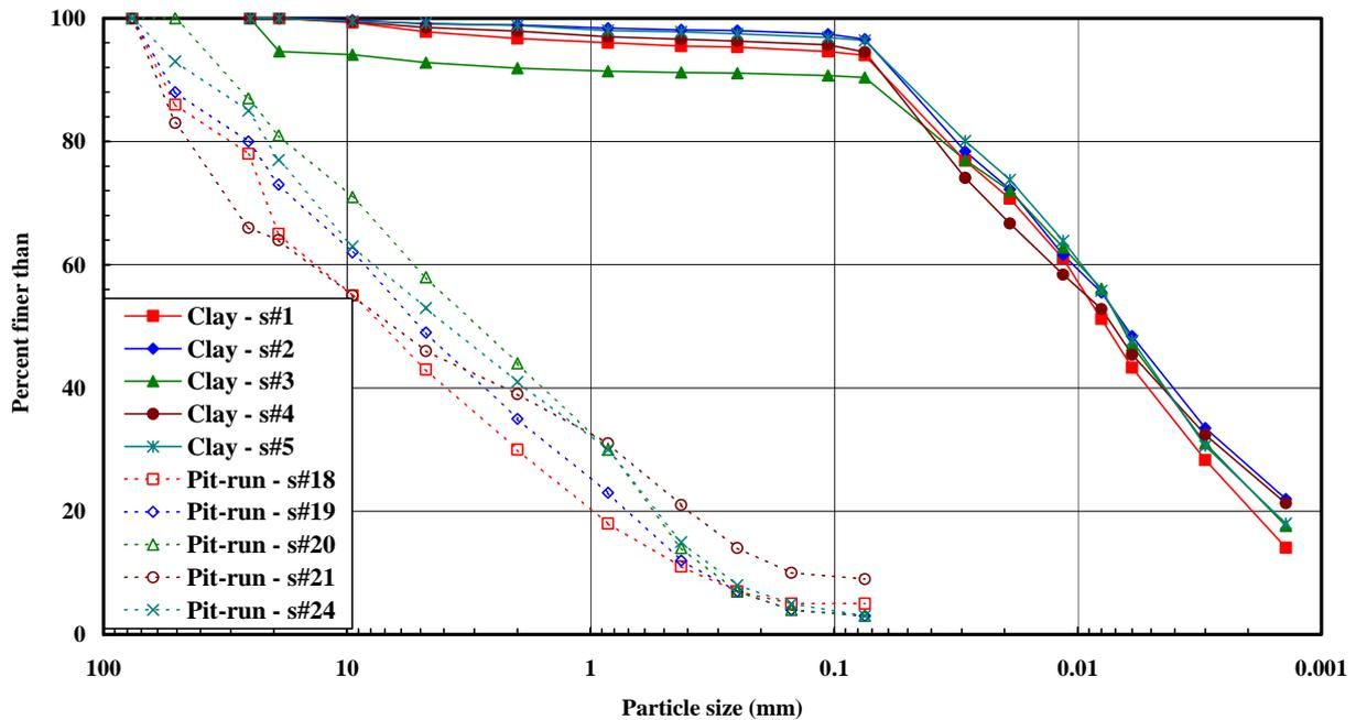
Figure 3. Particle size distribution of the Copper Cliff clay and granular growth medium material (pit-run).
