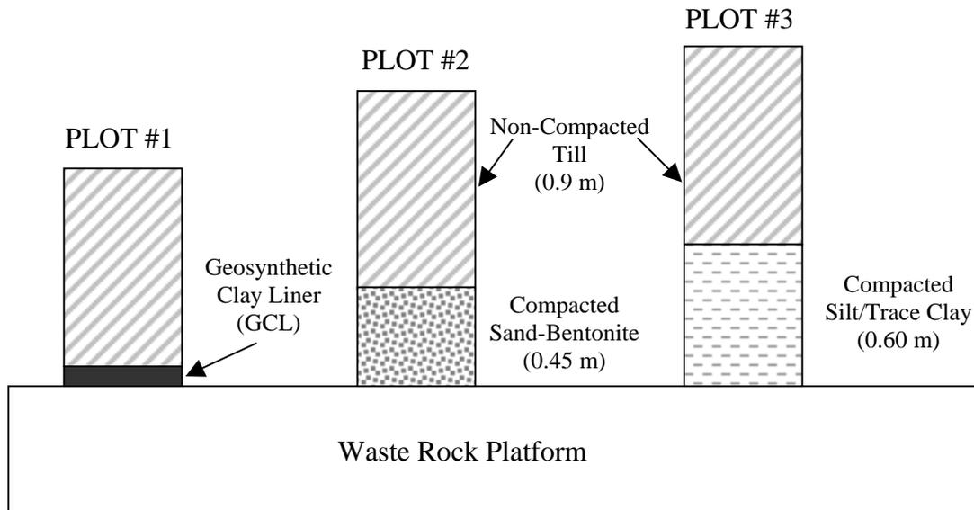
Figure 2. Schematic diagram of the Whistle Mine cover system field trials (from Ayres et al., 2002).
