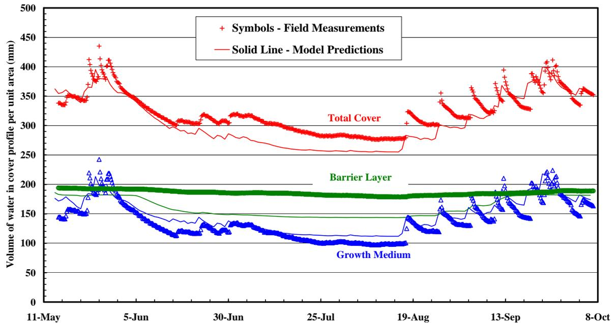
Figure 4. Cumulative water volume per unit area predicted and measured within each layer of the silt/trace clay barrier cover trial during unfrozen conditions in 2001 (from OKC, 2004).
