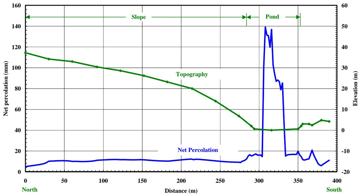
Figure 6. Predicted net percolation for the preferred cover design as a function of distance along the modelled cross-section for mean climate year conditions (from OKC, 2004).
