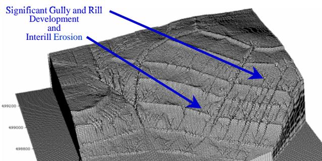
The second alternative and ultimate landform design implemented for the backfilled pit cover system consists of a number of catchments oriented parallel to the slope with a 'swale and ridge' pattern (see below). This micro-topography is beneficial for revegetation efforts because snow accumulates in the troughs, thereby increasing soil moisture levels, and wind velocities are reduced across
