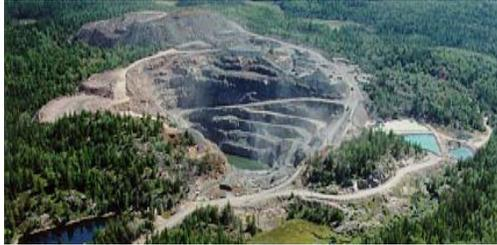
OKC completed erosion and landform evolution numerical modelling to design a runoff management system and final landform for the backfilled open pit at Whistle Mine near Sudbury, ON, Canada (Ayres *et al.*, 2007). The site has a mean annual precipitation and potential evaporation of 900 mm and 520 mm, respectively. Approximately 30% of the annual precipitation occurs as snow. Due to acid-
